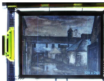
Figure 4: 4.1" AM-LCD with integrated IGZO semiconductor and AIPO dielectric
